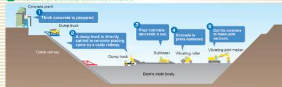
Construction of the RCD concrete method (1983)
