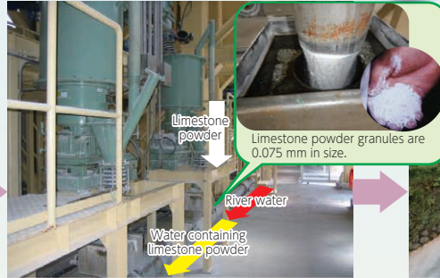
Limestone powder is mixed with acidic water drawn from the river
